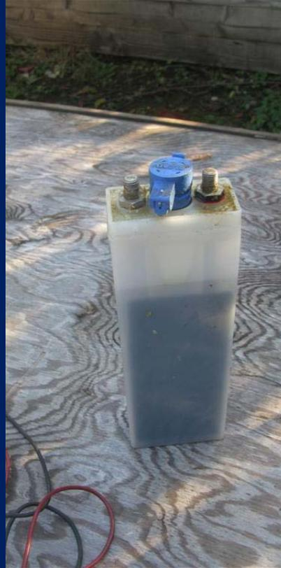
These 1.2 VDC, 10 amp single wet cell batteries were used for standby back up power. They have a 20-30 year life span and were replaced at about  $\frac{1}{2}$  their life span.
