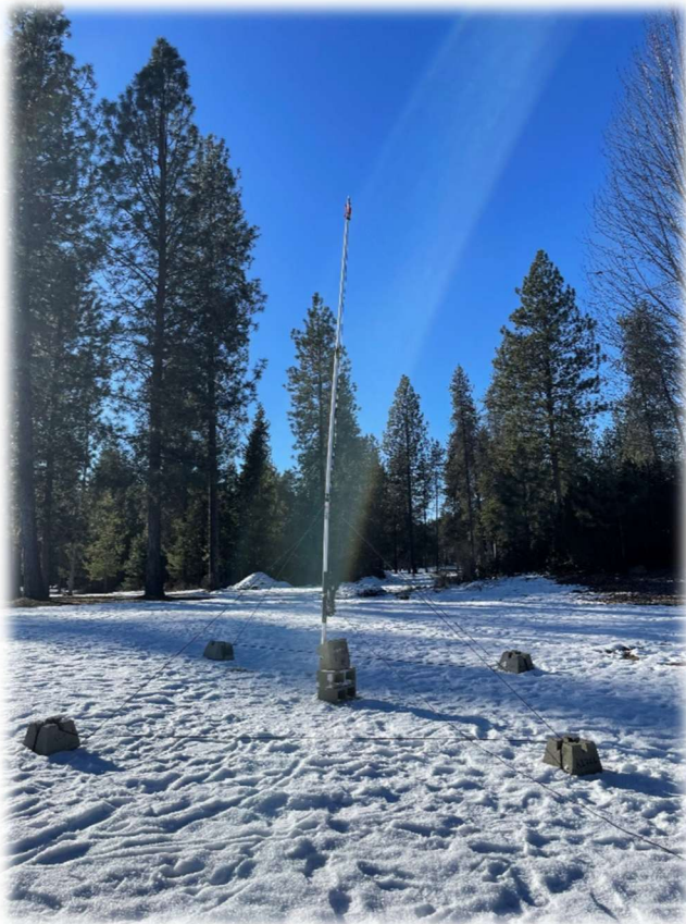
The antenna set up for Cynthia KI7AYR, an end-fed half wave.
