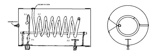
The can is made of 0.035 " copper sheet and the end caps are "oat meal box" type tops. The stiffener rod is 1/4 " fiberglass epoxied to the helix and supported on the end by copper wire loops made of # 12 copper wire soldered in place. The helix tuning is made of a copper penny soldered onto the end of a # 8 brass screw. The coupling loop is made of # 12 solid copper wire, which is fastened to the UHF connector on one end and the inside of the can on the other.
