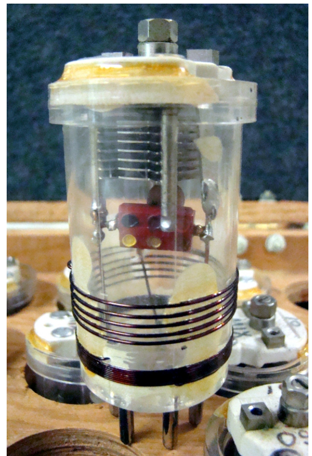
10 meter 5 prong coil detail - beautifully wound coils.
