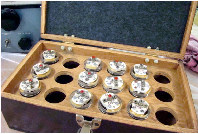
Coil storage box. 40 meter coils in receiver.
