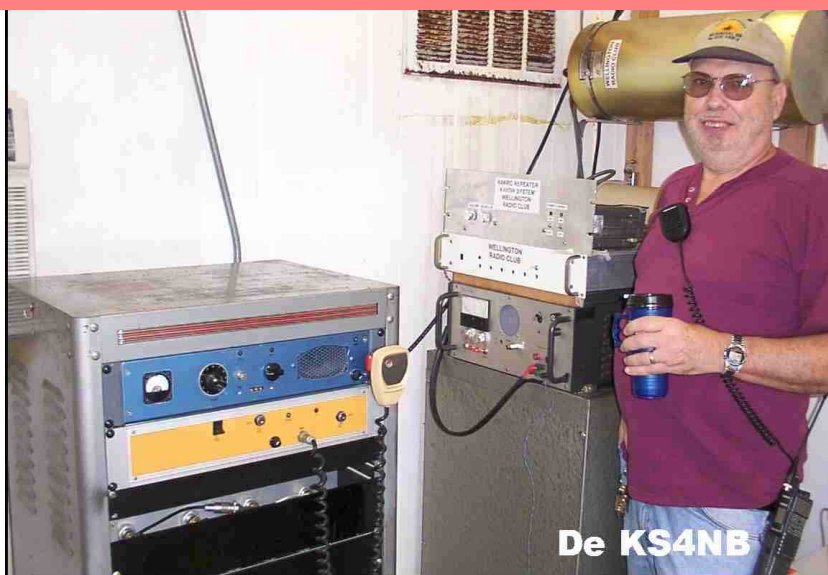
K4WRC-K4VOW REPEATER SITE A prime mover of the Repeater Committee, John WB4MOZ stands next to the two meter system... a converted GE MASTR Executive II, CAT 300 controller, Motorola power supply and Sinclair duplexor in cabinet. On the left is the 440 MHz repeater built and donated by John. Four other Village & FHP systems share the tower shelter.
