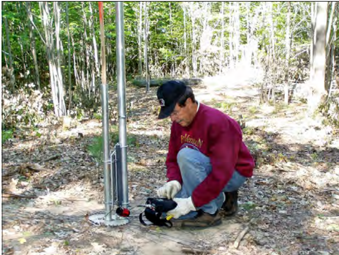
Tuning one of the 80 meter 4-square elements.
