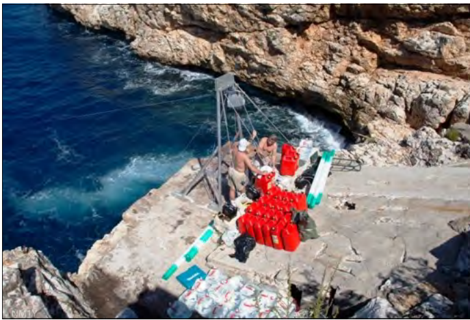
Mike N6MZ (r) and George AA7JV working the davit (designed and built by AA7JV) to bring ashore water, gasoline and other needed supplies carried on the Electra. The davit is 16m above the water.
