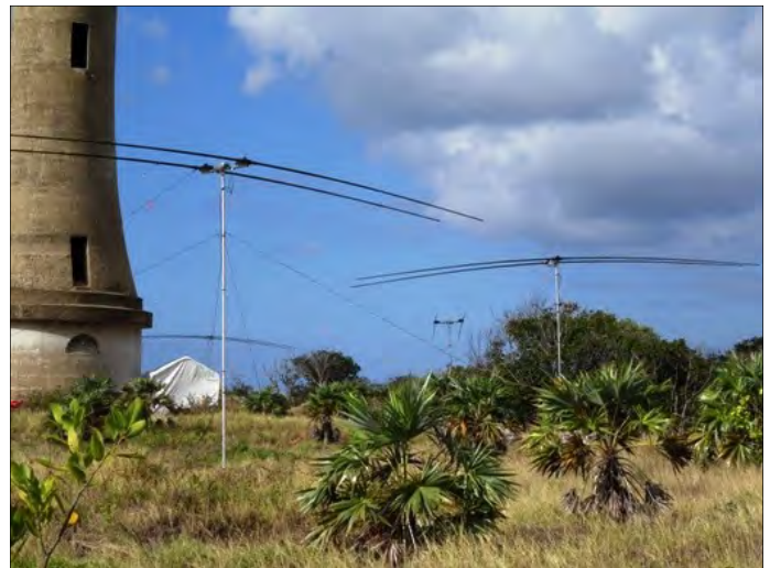
Four 2-element SteppIR beams on 7-meter masts.
