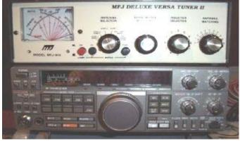
includes: Internal AT-440 Automatic Antenna Tuner: 80-10meters, 2.1KHz International Radio SSB filter, MFJ Deluxe Versa Tuner II model # MFJ-948: 160-10meters, Hand mike, Power cord, & Instruction manual with schematics
