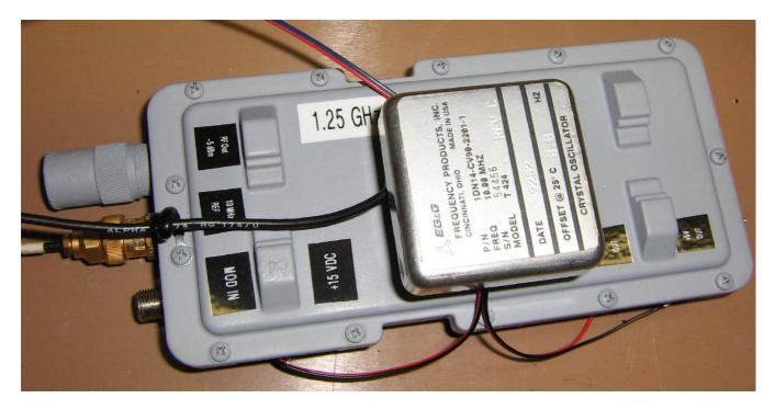
Attaching the external 10 MHz TXCO crystal to the outside of the MMDS downconverter case housing the oscillator board.
