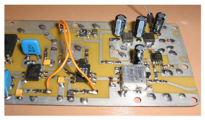
Constructing the 1.25 GHz phase–locked loop oscillator board.
