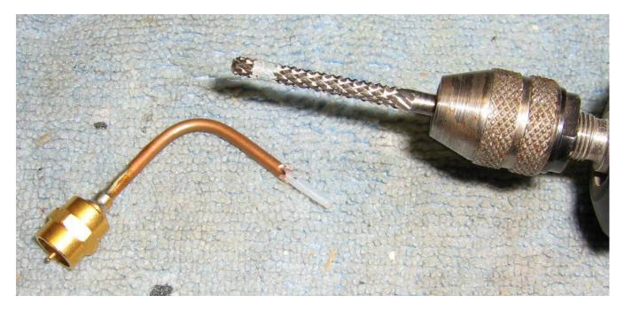
Use a Dremel tool with a drywall bit to grind away *just* the copper jacket of the UT-085 semi-rigid coax, leaving the Teflon dielectric exposed.
