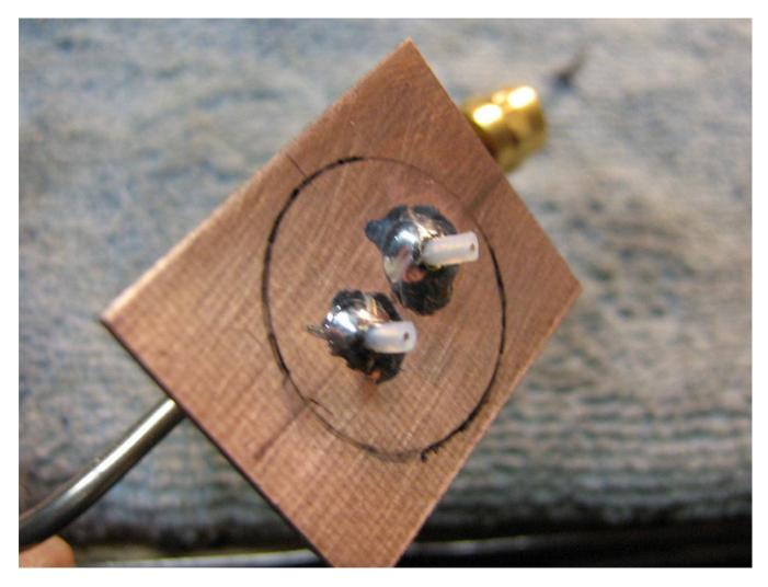
Solder the two pieces of UT–085 semi–rigid coax into the holes you drilled and then trim the two Teflon–coated "probes" so they are only 5/32–inch above the PC board. Use as little solder as possible to hold the probes. Solder is quite lossy at 10 GHz.
