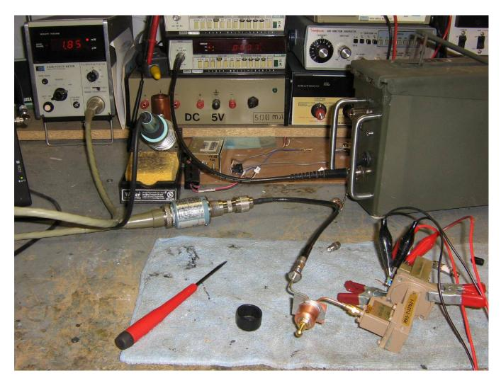
Testing and tuning the finished bandpass filter. The filter's insertion will be around 1 to 2 dB, depending on the cavity's "Q" and coupling probe lengths.
