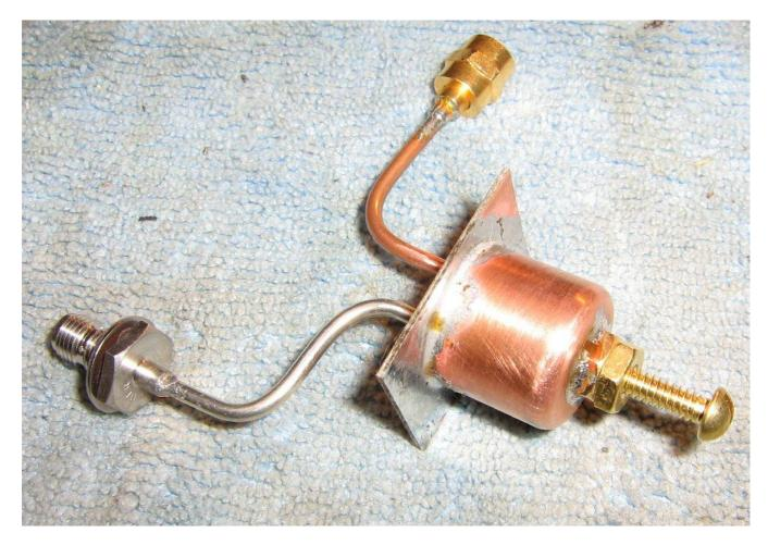
Overall view of the finished copper pipe end cap bandpass filter.
