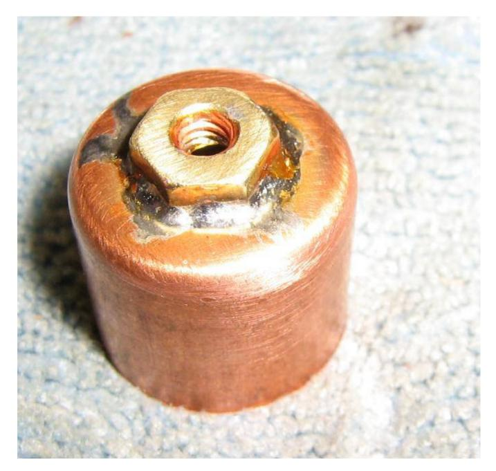
Clean up the copper pipe end cap and nut from any excess solder using a piece of emory cloth.
