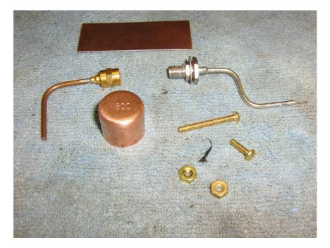
All the parts you'll need to construct a 10.5 GHz bandpass filter. That's it!
