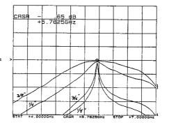
1/2 Inch Filter: Again I noticed how far down in frequency the filter tuned. A slightly longer screw protuding about  $1/2^n$  into the filter resonated on 5760 MHz. I don't have a family of bandpass plots a 5.7 GHz, but the Q's were very high and the skirts quite steep.
