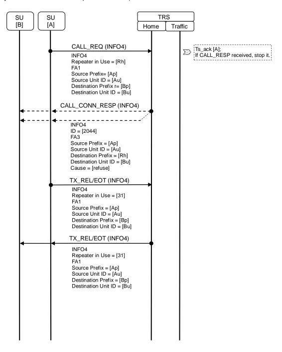
Figure 18.2-3 Sequence Diagram for Link refuse
