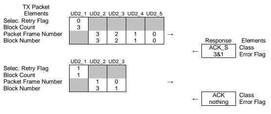
Figure 12.4-1 Information elements configuration for Selective Retry
