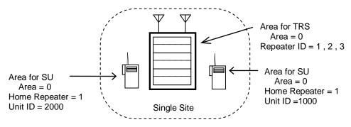
Figure 4.1-1 Concept configuration of Single Trunked System
