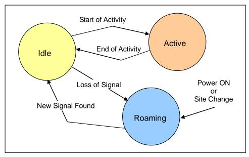
Figure 6.1-1 Basic Data Flow for Roaming Process
