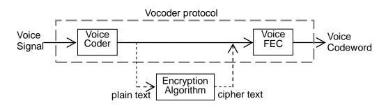
Figure 16.2-1 Encryption Processing Diagram
