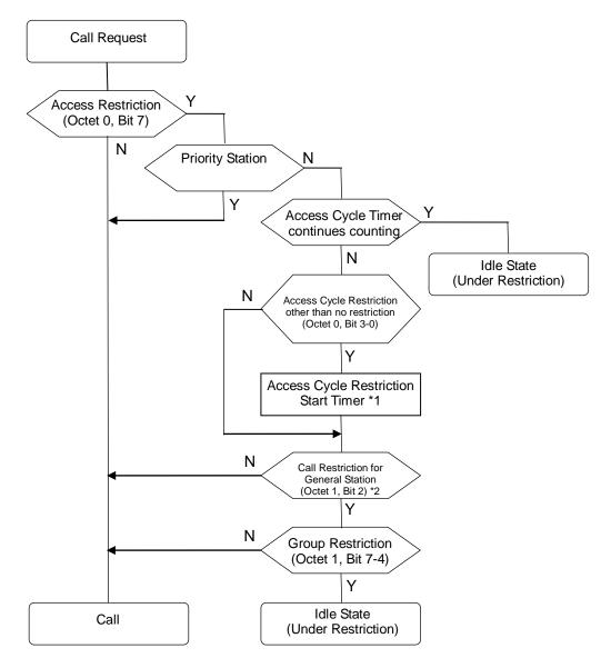
\*1 The timer expires when the duration configured for access cycle intervals elapses. \*2 The case of a location registration request, the location registration restriction for a general mobile station (Octet 1. Bit 3) is applied.
