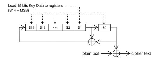
Figure 16.3-1 Scramble Encryption Algorithm
