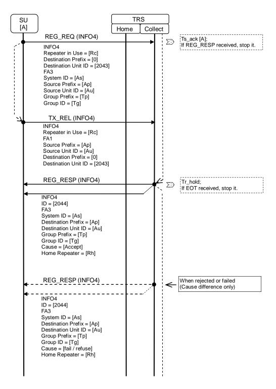
Figure 18.3-2 Sequence Diagram for Registration - 2
