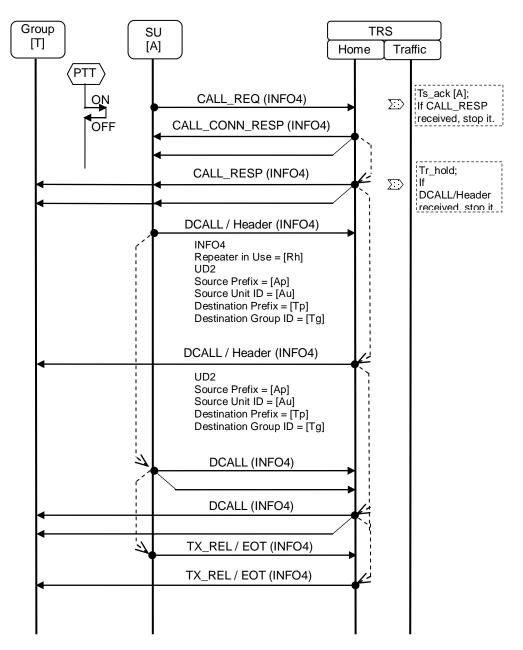
Figure 18.15-1 Sequence Diagram for Broadcast Data Call
