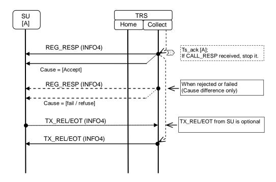
Figure 18.7-2 Sequence Diagram for Authentication during Registration - 2
