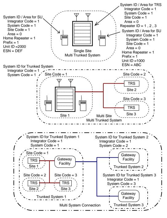
Figure 4.1-2 Concept configuration of Multi Trunked System
