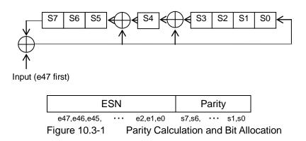
The Authentication Value is obtained by a bit scramble processing using an exclusive-or operation among the 56-bit data sequence and the data sequence of a polynomial P(x). Figure 10.3-2 shows the bit scramble processing.
