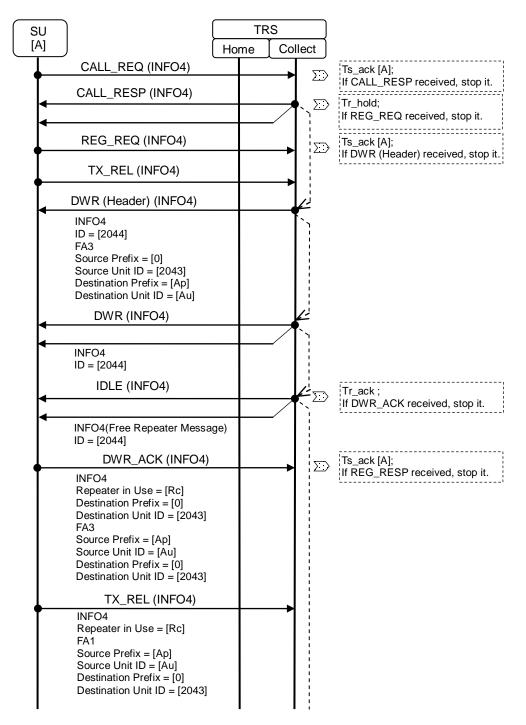
Figure 18.9-1 Sequence Diagram for System Data Write during Registration - 1
