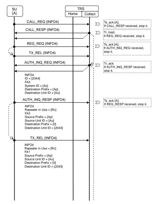
Figure 18.7-1 Sequence Diagram for Authentication during Registration - 1
