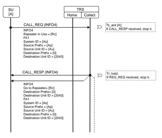
Figure 18.3-1 Sequence Diagram for Registration - 1
