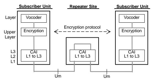
Figure 16.1-1 Layer for Encryption Protocol
