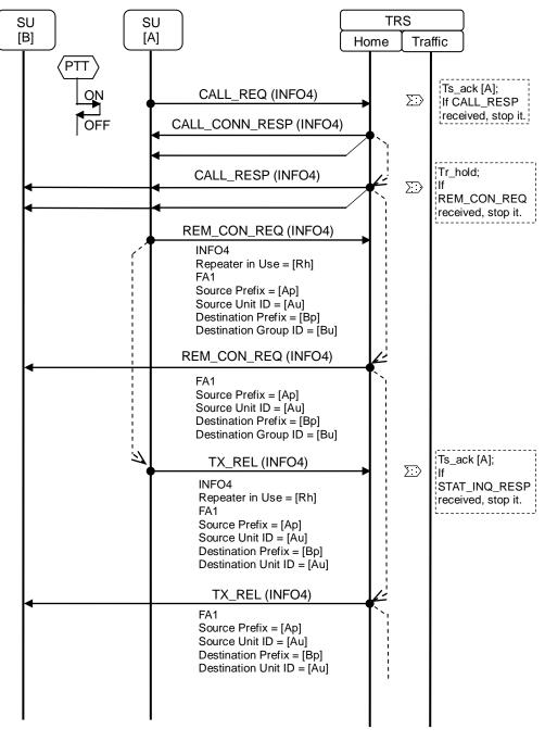
Figure 18.23-1 Sequence Diagram for Remote Monitor – 1
