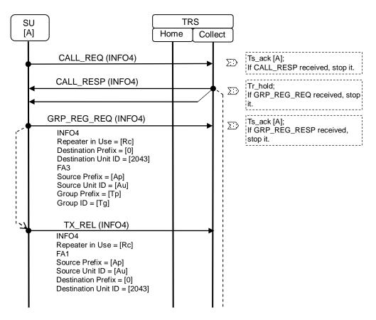
Figure 18.6-1 Sequence Diagram for Group Registration - 1
