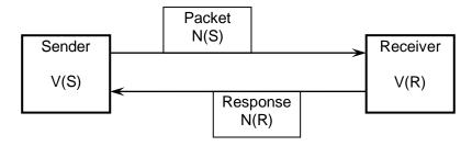
Figure 12.3-1 Conceptual diagram of packet synchronism
