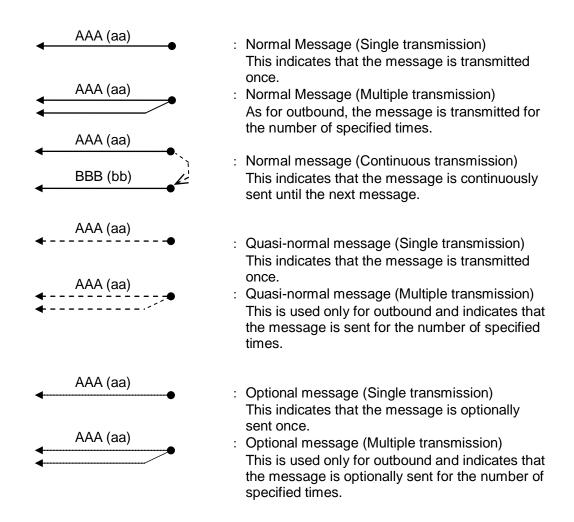
In notation of XXX (xx), "XXX" represents the name of abbreviated layer 3 message and "xx" represents the name of a functional channel (SCCH Messages). The solid line represents a normal message that is always used in each procedure.
