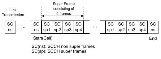
Figure 11.1-1 Frames Structure for Voice Call
