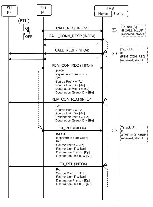
Figure 18.22-1 Sequence Diagram for Remote Stun - 1
