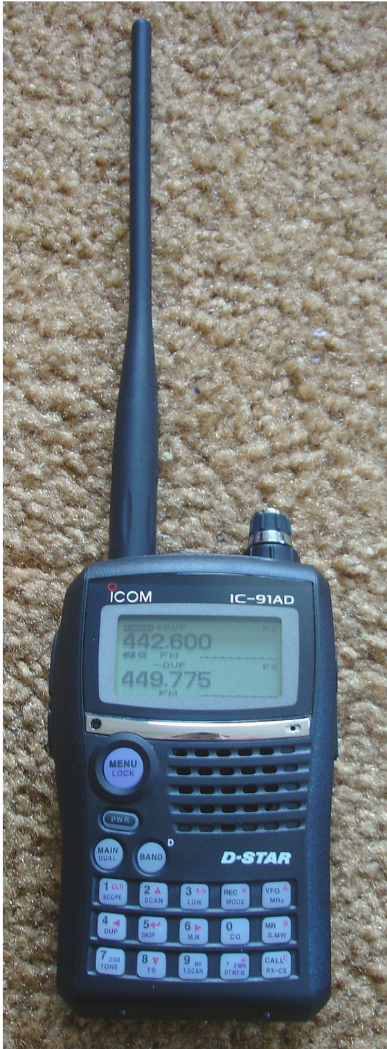
ICOM IC-91AD handheld transceiver with the D-STAR UT-121 digital voice board installed
