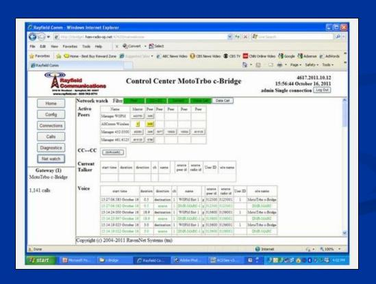
■Built-In Diagnostics for troubleshooting IP network problems and monitoring system operation
