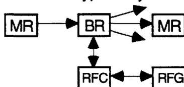
Figure 8-1 Data System with Asymmetrical Addressing
