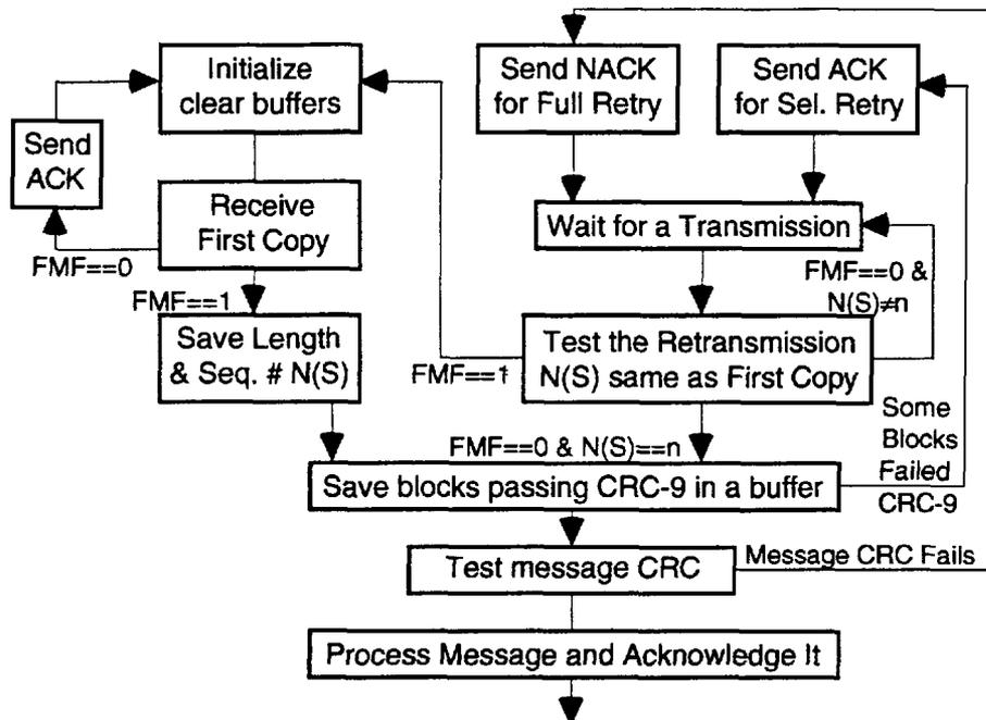
Figure 9-1 Confirmed Delivery Packet Reception State Diagram
