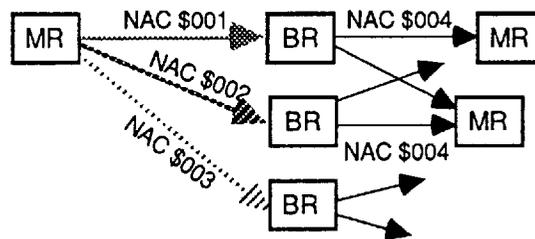
Figure 3-1 Separated Repeaters Servicing a Wide Area
