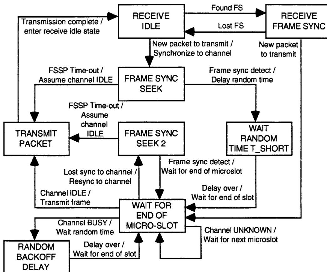
Figure 8-2 Channel Access State Diagram
