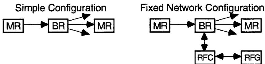
Figure 7-1 Repeater Configurations
