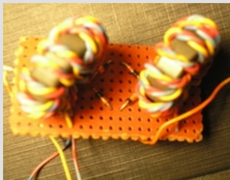
Fig. 8 - Mixer Circuit (2 Required)
