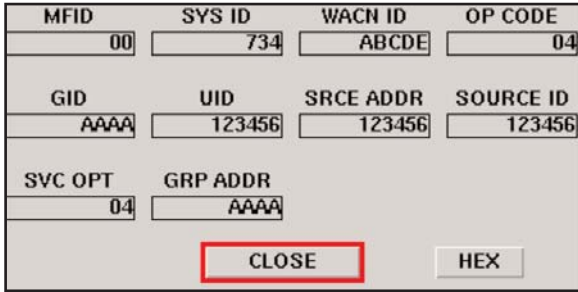
Figure 37: The P25 Trunking Uplink Configuration Decode Screen.
