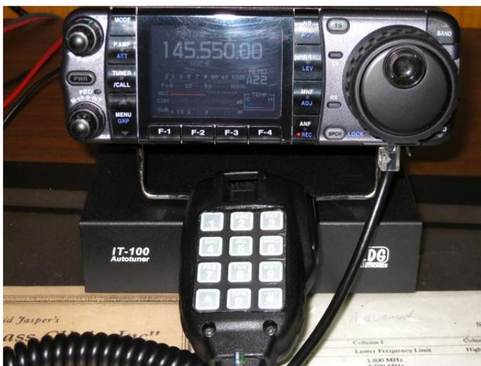
DTMF pad installed. Black silicone fills opening around pad
