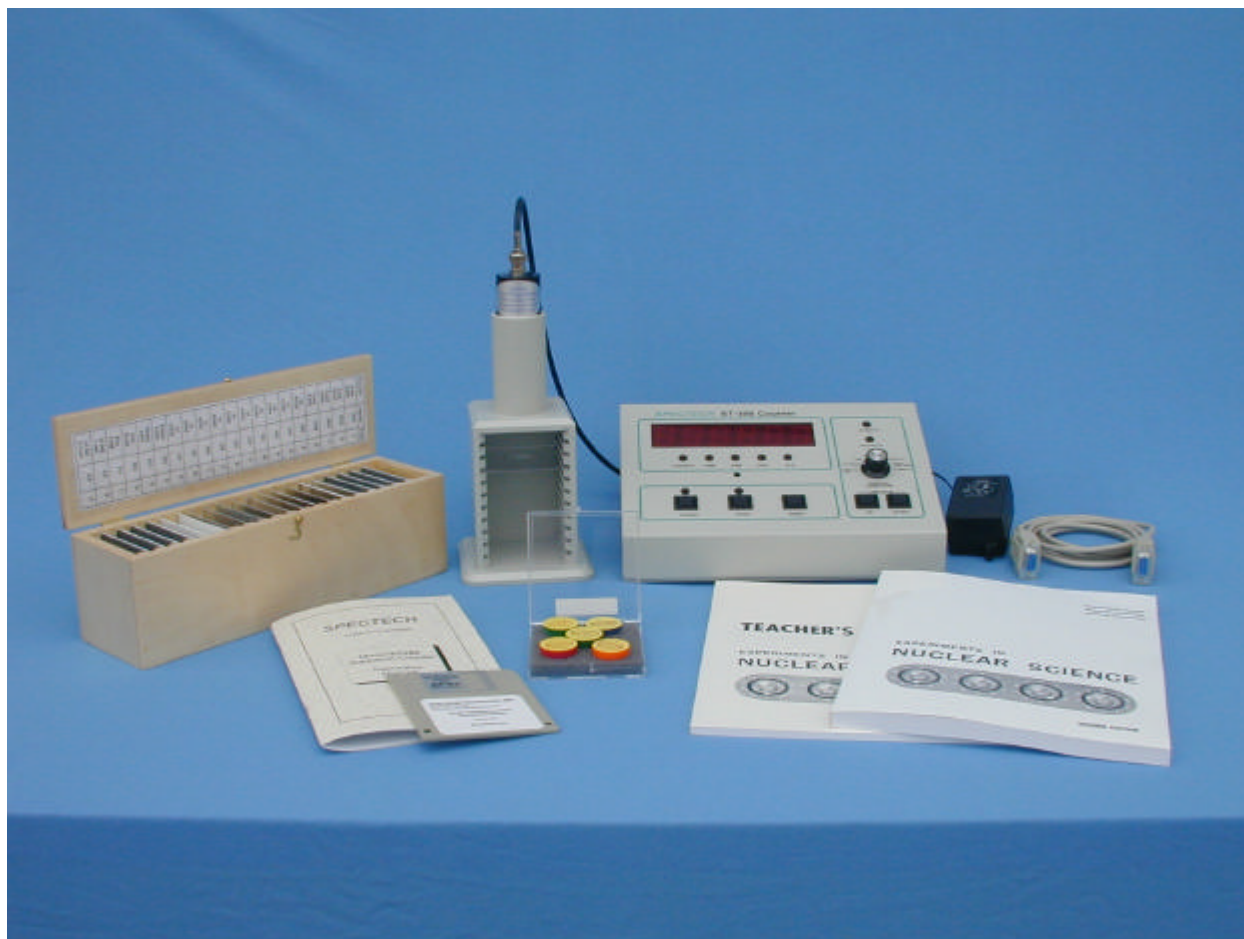
Figure 2: Setup for ST350 with sources and absorber kit.
