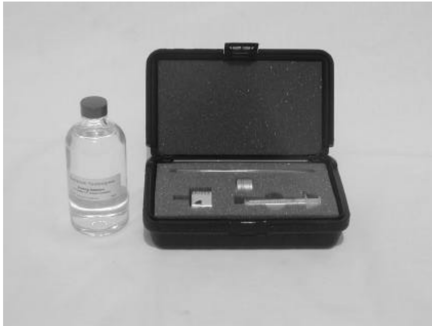
Figure 3: Isotope Generator to make Ba-137m from Cs-137
