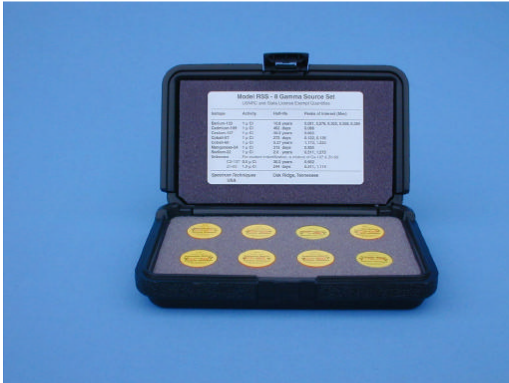
Figure 3: Kit of eight different gamma sources.
