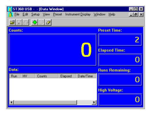
In the upper part of the main display are the menu headings. From left to right, they are: *File*, *Edit*, *Setup*, *View*, *Preset*, *Instrument Display*, *Window*, and *Help*. Menu selection is either by using the mouse or by holding the *Alt* key and pressing the key corresponding to the underlined letter in the title's name.
