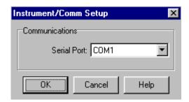
After switching COM ports, click on ReSync under the Setup menu to re-establish communication. If communication will still not re-establish, check for an improperly connected or defective serial cable.
