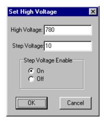
The *High Voltage* and *Step Voltage* values are displayed in the lower right corner of the main display. If the *Step Voltage Enable* is set to *OFF*, only the *High Voltage* will be displayed.
