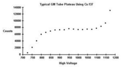
Notice that the counts form a relatively flat place on the graph between 850 and 1100 volts. The center of this area, at approximately 1000 volts, is the recommended operating voltage for the detector. However, any voltage in this flat region would be acceptable. Also, notice that the counts increase rapidly as the high voltage nears its upper limit. This indicates that the tube is entering its breakdown region. Do not continue to operate the tube in this region.
