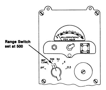
(2) Listen to clicks in the headset and/or observe the meter indications while approaching the suspected radioactive area or object. If the needle on the indicating meter does not move above 50 mr/hr (one division on the scale) then move the range switch to the next lower scale.
