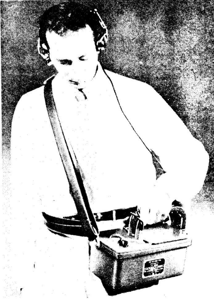
Fig. 3-4 Survey Meter AN/PDR-27A showing attachment with shoulder harness.
