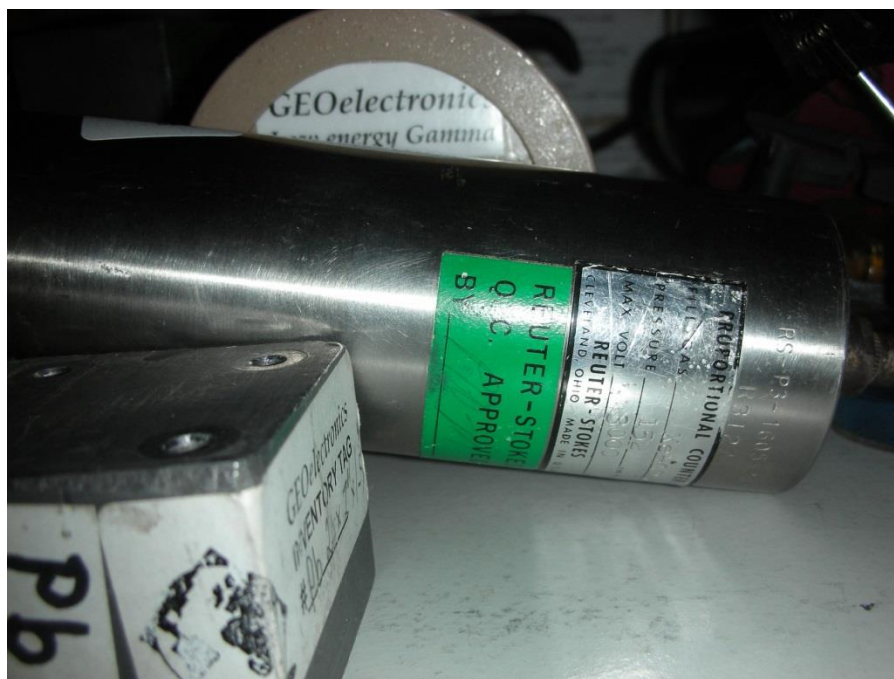
A sealed Xenon gas proportional detector tube. XRF taken through its Beryllium window.
