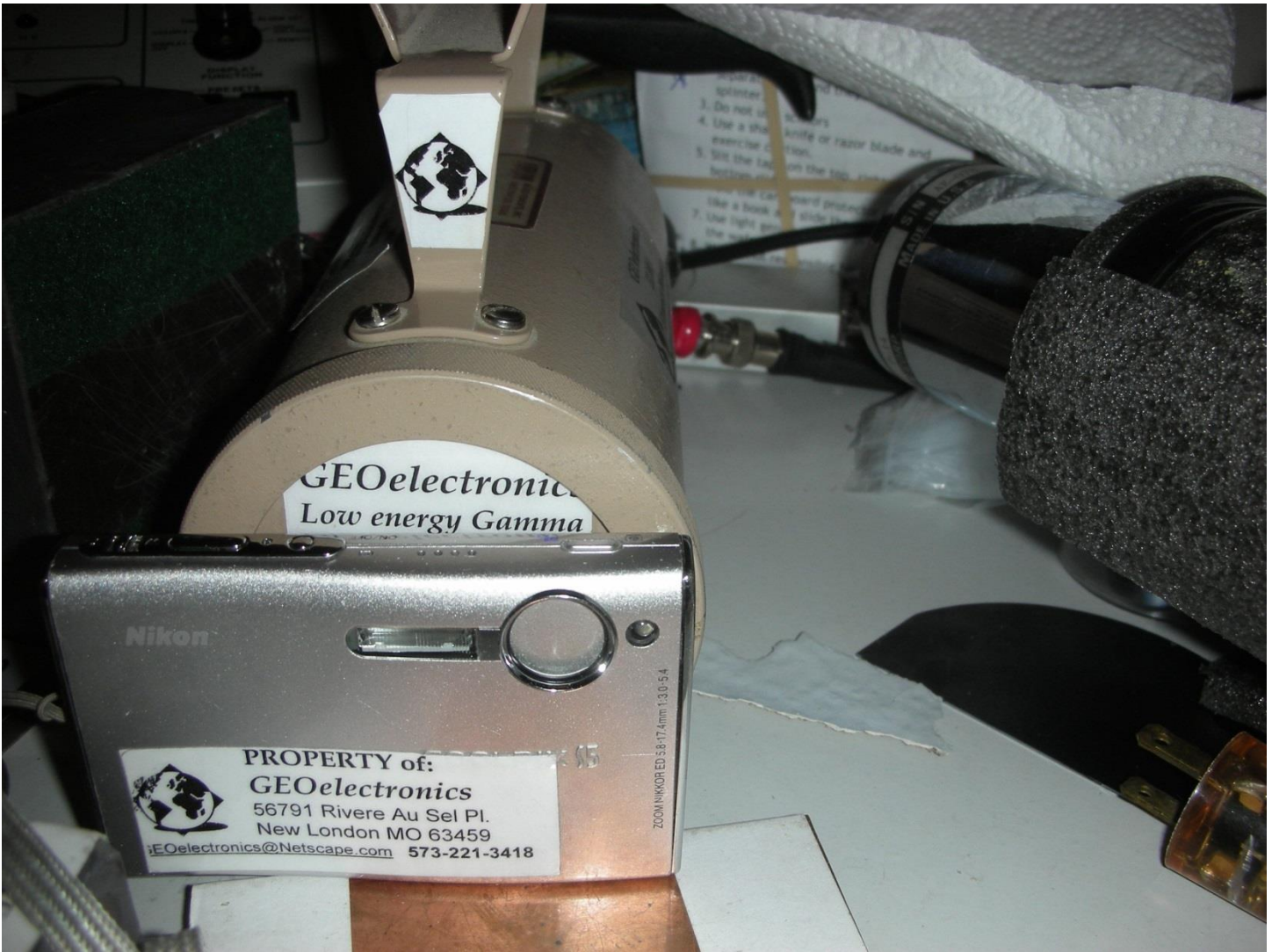
Testing a digital camera TFT LCD display for lead and rare earths.
