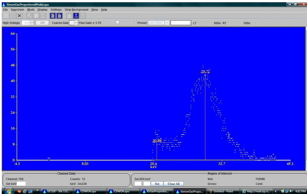
A sealed Xenon gas proportional detector tube. XRF taken through its Beryllium window.
