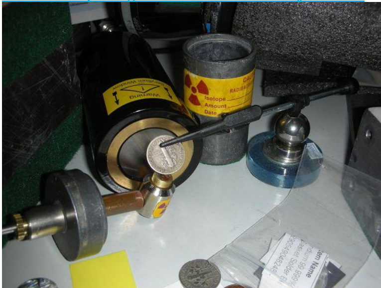
FIG. 7> Setup using old US dime coin to test for silver:
