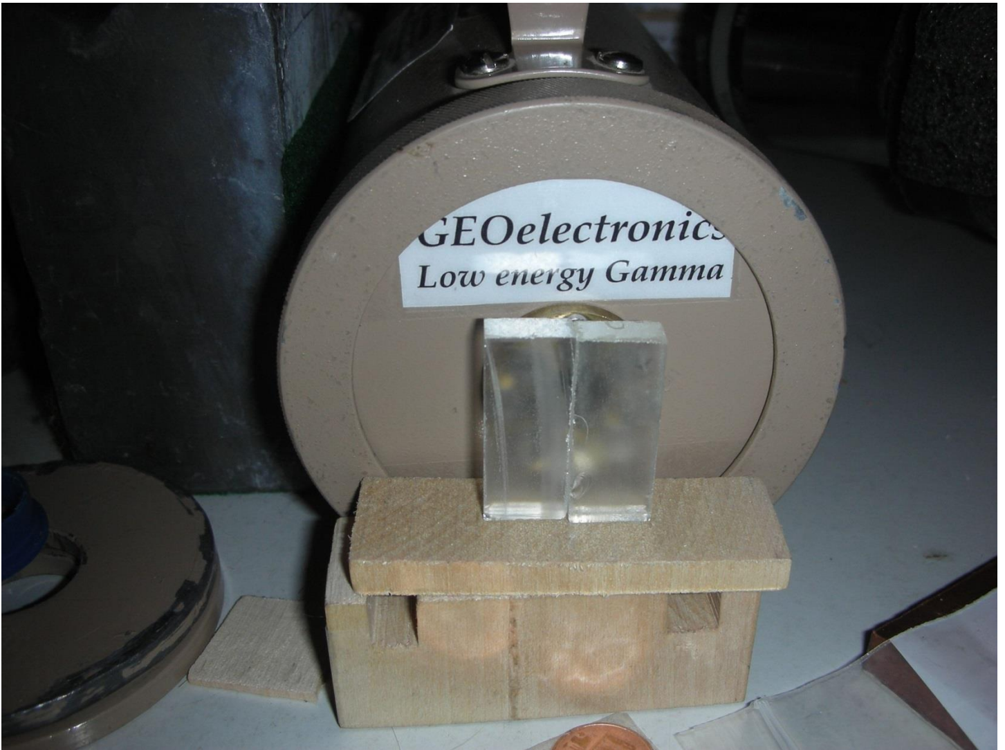
BGO Crystals (Hospital PET-CT Scanner sensors)
