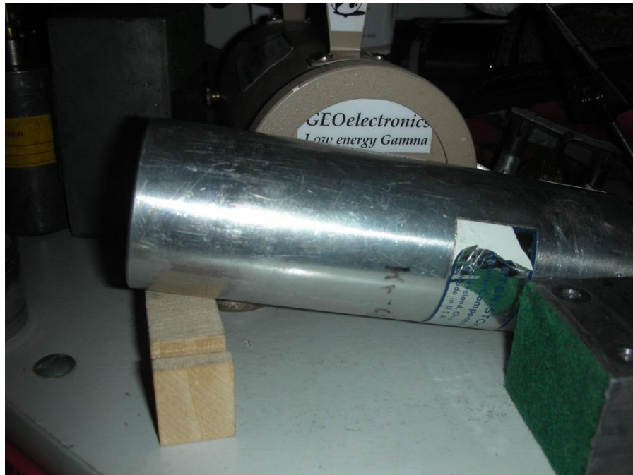
A Krypton Gas proportional detector tube, with Beryllium window.
