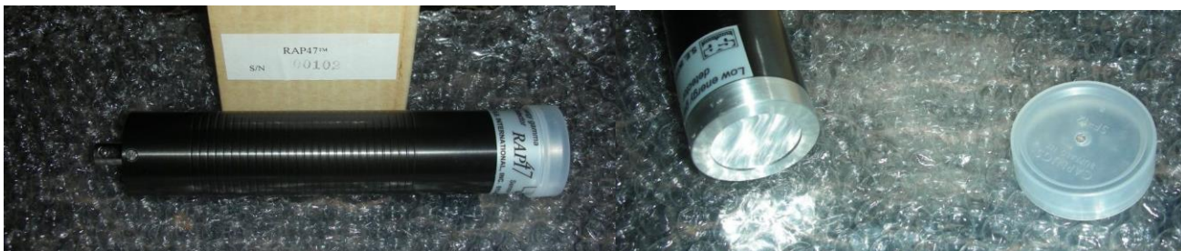
FIG.2>Rap-47 1" Diameter Low Energy Probe: FIG.3>RAP-47 1" thin aluminum window and protective cap:
