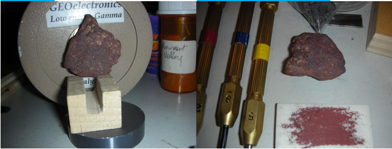
FIG.12A> APXS/XRF definitely show red rock does test positive for iron!
