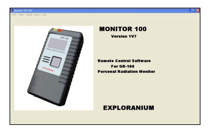
Four menu items are available in the menu bar, three of which are for controlling the unit: Tests, Setting and History. The Exit button stops the program. To switch among the Tests, Setting and History screens, you have to return to the main menu first by clicking on the Main Menu Button.
