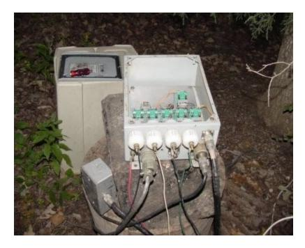
Before going into the main coax to the shack (also Triax), we pass through a BCB filter and preamp designed for 75 I/O and powerfed up the feedline. From the output, the cable travels about 300 feet into the shack areas and is terminated at the main Bulkhead/Patchpanel. A MIL E rated connector allows quick disconnect of the control wiring, in case of service. Of course the short groundwire is attached directly to a brass stud on the box.
