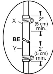
**NOTE:** When installing BE tube, ensure at least 2" (5 cm) length of the adjoining 3/4" (1.9 cm) tubes are inserted into R7000BE (Figure A, points X and Y).
