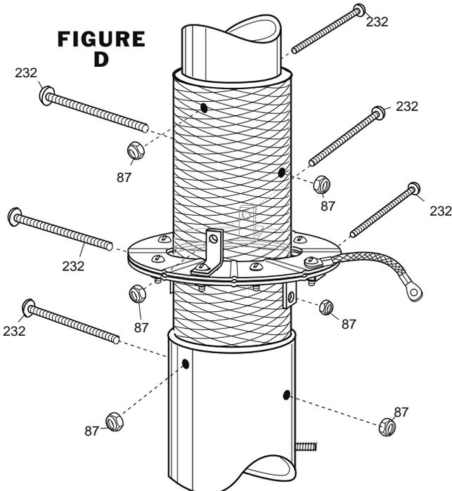
Figures A through D show the steps for radial ring assembly. Refer to the Radial Ring Subassembly Parts List for the parts required in this step. Attach the rings(74) to the base using the radial ring brackets (73), 2-1/2" (6.3 cm) screws (232), 1/2" (1.3 cm) screws (79) and lock nuts (87). Leave hardware loose until Step #2. Note the proper orientation of the radial ring brackets in Figure A. Install jumper strap (428) as shown in Figure D.
