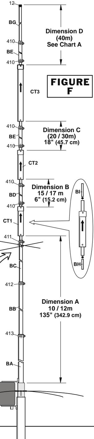
Secure hose clamps about 1/4" from top of each slotted tube to ensure adequate compression.
