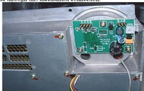
IC-EX243px board mounted in IC-735 Beneath the Speaker on the PA Unit.
