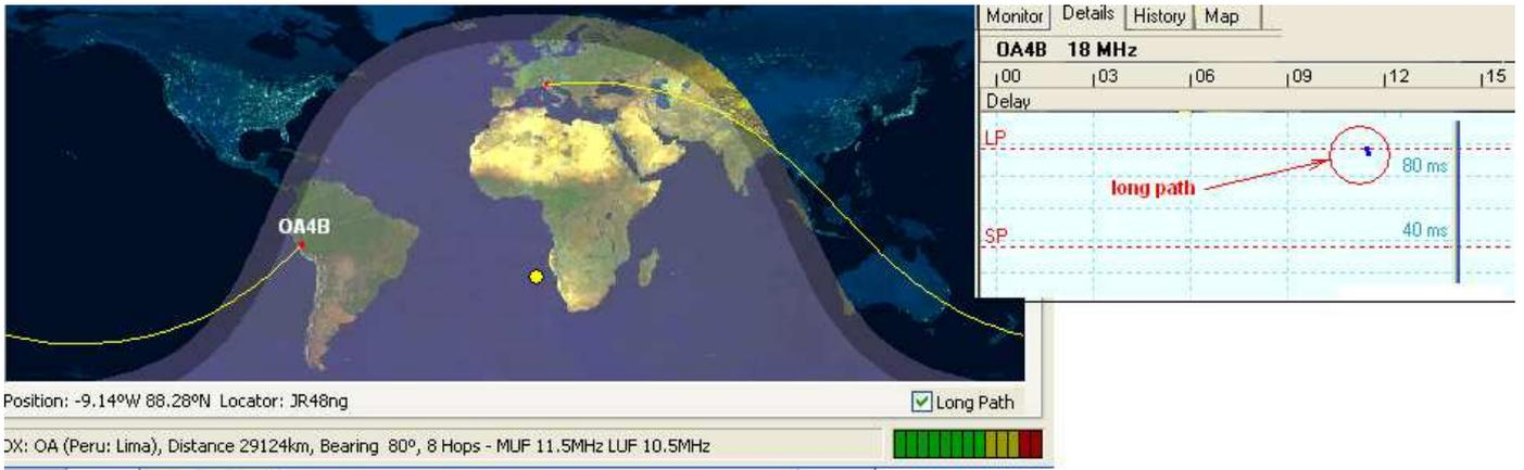
spectrographic analysis of the received signal made with the software spectrum lab in order to shows a trace of multi-path, the signal coming from both directions.
