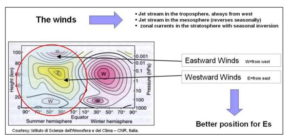
These winds, which are active most days for part of the day, cause Travelling Ionospheric Disturbancies (TIDs) which result in fluctuations of electron density and formation of amasses.
