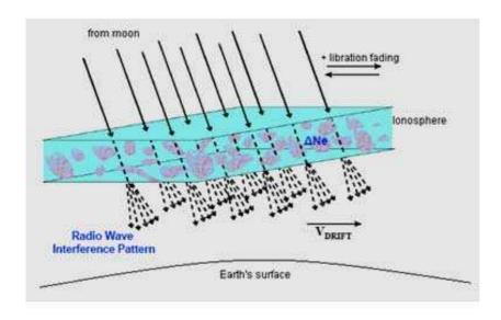
Rapid scintillations caused by ionospheric irregularities (ssTIDs, periods of some minutes)
