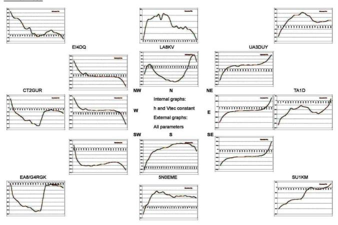
In order to separate the eventual tendencies from changes in the ionosphere (which occur over a full moon pass, but are negligible in a short period), we computed also the rotations with constant VTEC and slab thickness, i.e. for an invariable ionosphere.
