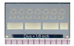
The LED Display will fit either way round, either with the bargraph above or below the Digital display.
