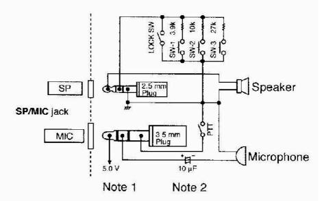
**Note 1:** Voltage is developed across a  $100\Omega$  resistor on the 5 V line in the transceiver. When 2 mA flows, approximately 4.8 V is developed.
