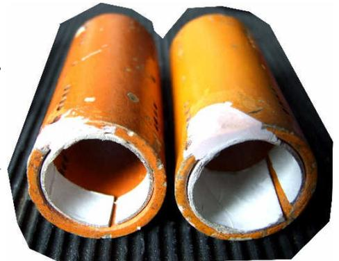
Two of the ceramic formers has bits missing, the usual chips etc around one of the mounting holes where some dip stick had over tightened the mounting. I used P38 car body filler to refill the missing bits, a cardboard tube inserted inside the former to hold the new bit in place.
