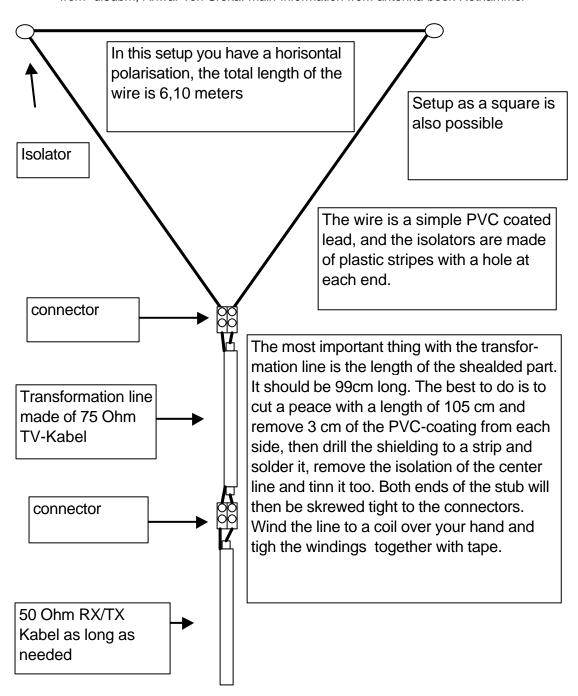
I put up the antenna in the loft, the antenna worked well from the beginning. Dipending on the surroundings you might have to tune it, by changing the length of the radiating wire. I worked a lot of stations with this antenna!
