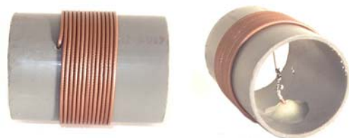
80m Coax Trap before sealing
