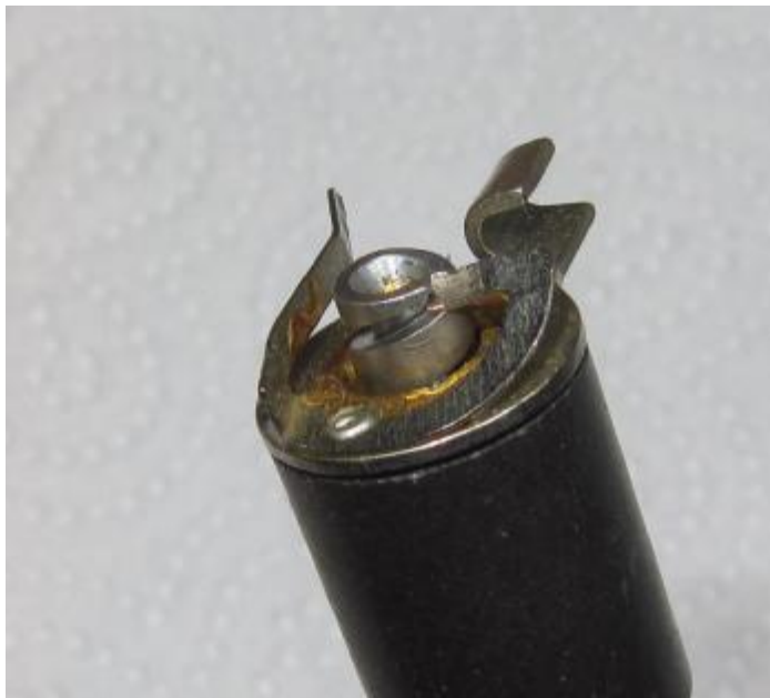
Fig. 4 Metal and spring assembly at the PTO core
