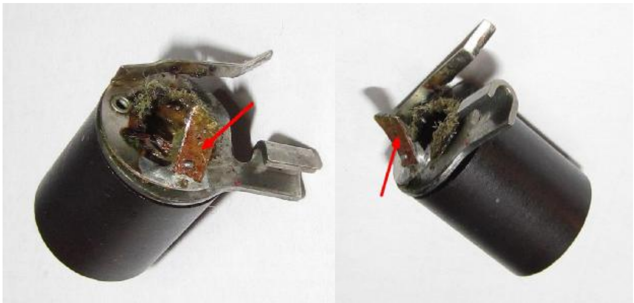
Fig. 1 damaged spring assembly at the PTO core
