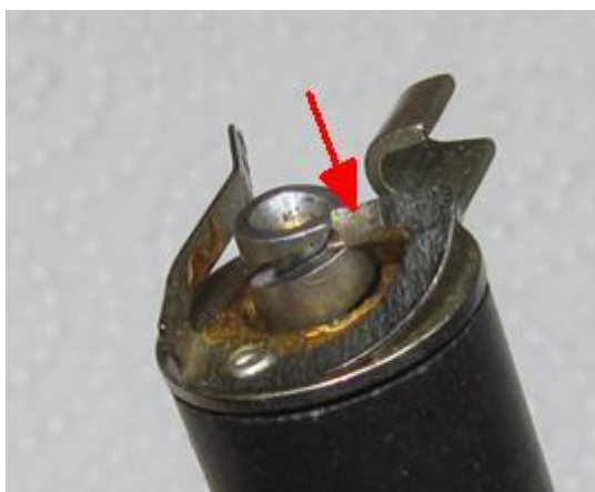
Fig. 2 undamaged spring assembly at another PTO core
