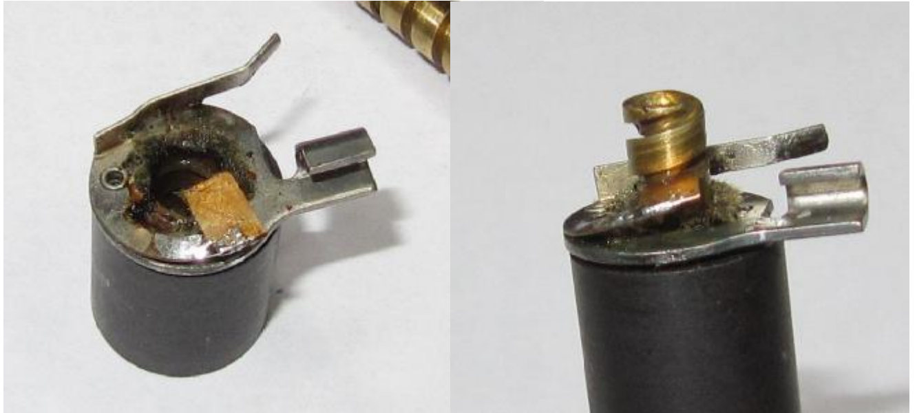
Fig. 3 repaired spring assembly at the PTO core
