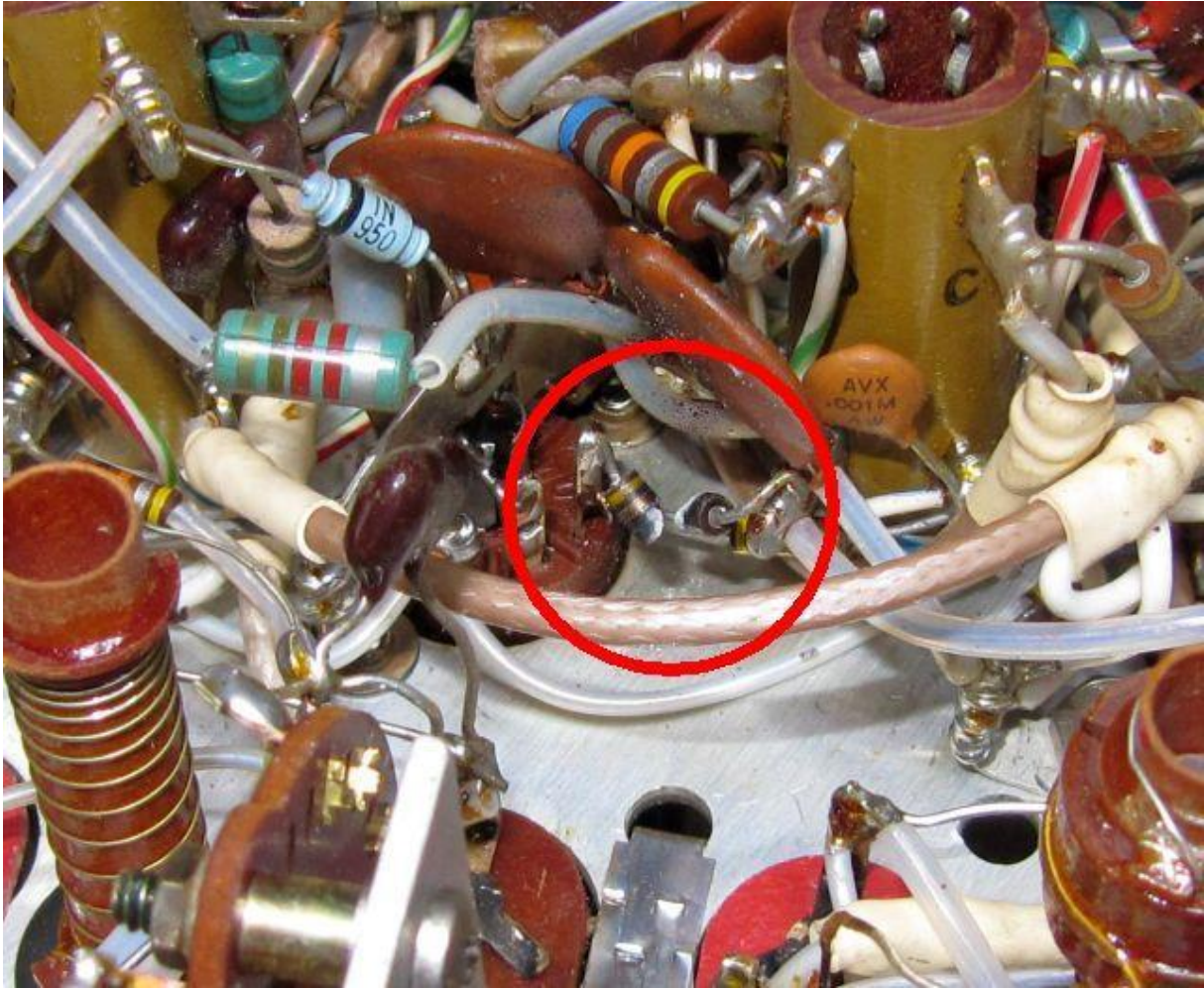
Fig. 1: The broken resistor R9 at pin 1 of V7 (RF shields removed)
