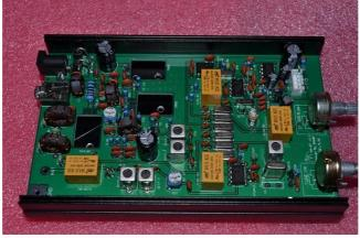
[ ] Bend the pins of the 7808, IRF640, and D882 semiconductors as shown. Please note that IRF640 is a electrostatic sensitive part, so handle it with care.
