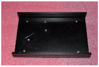
Install the 4x rubber feet with 4 pairs of M3x10 screws and M3 nuts.
