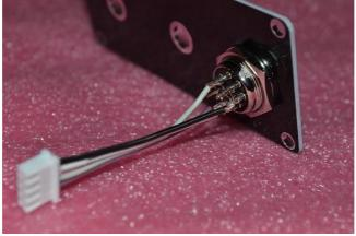
[ ] Plug in the microphone cable into the SIP4 socket on board, install the front panel using two black chassis screws, then install the knobs.
