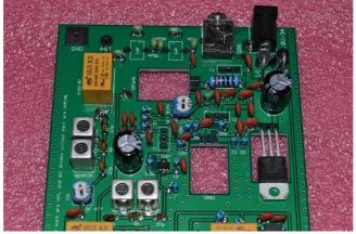
Desolder the 7808 voltage regulator, and clean the solder from the pads and pins
