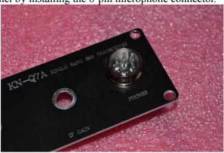
[ ] Solder the microphone cable, based on the schematic below. This connection is compatible with ICOM HM-series and the supplied optional microphone. To use a different brand microphone, please identify the pinout and wire it accordingly. On the SIP4 connector pin 1 is +8 V, pin 2 is PTT, pin 3 is MIC, and pin 4 is GND.
