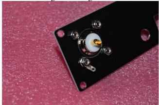
[ ] Install the rear panel using two black chassis screws and solder the antenna connector.
