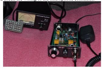
Setting bias voltage for the final amplifier IRF640: Connect an ampere meter in series with the power cable (set to measure 1A or more), press PTT but **do not talk to the microphone**, the current will likely be 0.48 A. Then turn SET BIAS trimmer clockwise SLOWLY until the current increases 60mA to about 0.54 A. Note that, if you turn the trimmer too quickly, or the preset position is not in the middle, the IRF640 might conduct completely and it may cause an over current failure.
