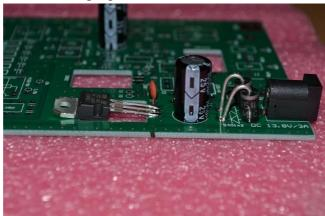
[ ] Plug in a 12~13.8 V power supply and measure the voltage on pin 3 of 7808 near to the 104 capacitor to see if it is within +/-5 % of 8 V; if not, check power supply polarity and your soldering [ ] Disconnect the power supply and proceed to the next step.
