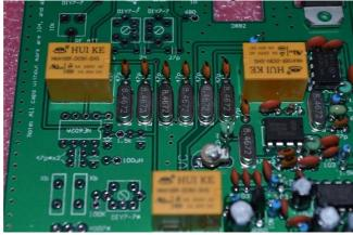
[ ] Plug in a 12~13.8 V power supply and connect an external speaker to the speaker connector. Touch pin 5 (not pin 2) of the uninstalled NE602A using tweezers to note a little noise from the speaker. If it is not normal, please check your soldering. If it is okay, disconnect the power supply and the external speaker to proceed to the next step.
