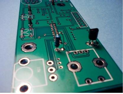
Fit push buttons, encoder, volume control, microphone connectors in place, and solder. For LCD, you may need to scratch the pads to make sure it is shining, so you can solder it well. Find M3x4 screws and install two copper standoffs.
