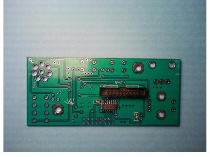
Solder small parts on top layer (component layer) first. For 1k resistor, it is suggested you solder on top layer as shown, if not, you may melt the plastic on IDC connector. For diodes, use 1N4148, and pay attention to polarity.
