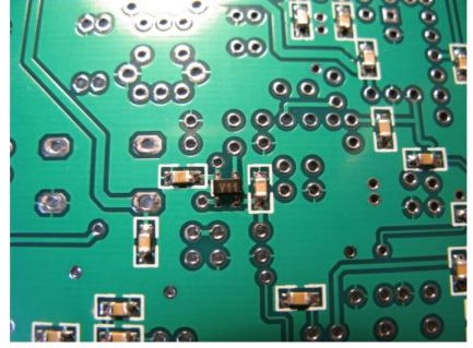
Solder DDS chip carefully on top layer (component layer). If you don't have experience soldering SMD IC, please find some readings and read it carefully. Or more wisely, ask experienced guys for help. This chip is expensive and weak, so do it carefully and slowly. You can see some pins are connected together, never mind, this is by design to have 4 pins connected on one side, and 2 pins on another.
