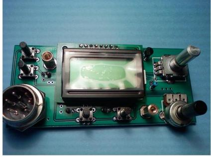
Put on black front panel and check the locations of push buttons, controls to extrude out properly, and this is the end of the simplest board installation. There is no way to apply power supply to do some actual smoke test now. Enjoy the completed work, and stay tuned.
