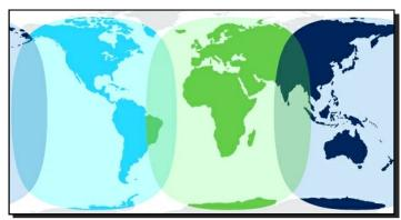
**Showing BGAN Coverage Using 3 Satellites**
