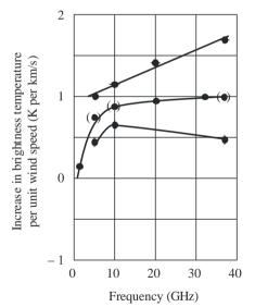
c) Spectrum of increase in brightness temperature caused by wind at the ocean surface
