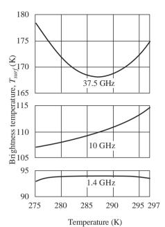
b) Brightness temperature of the sea surface as a function of sea surface temperature (nadir) for a salinity of 36 parts per thousand
