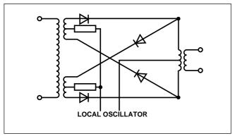
Fig. 10 Resistive loaded high intercept point mixer
