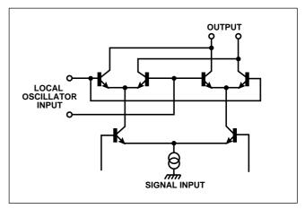
Fig. 13 The transistor tree
