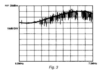
The amplitude relationships of the third order intermodulation products and the fundamental tones may be derived from Ref.1, where it is shown that the intermodulation product amplitude is proportional to the cube of the input signal level. Thus an increase of 3dB in input level will produce an increase
