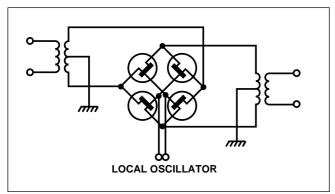
Fig. 11 Quad MOSFET commutative mixer
