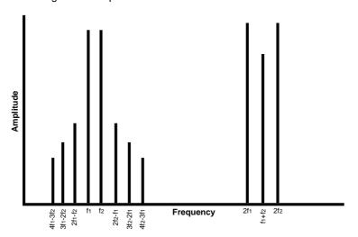
Fig. 1 Intermodulation Products
