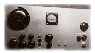
Homebrew 20-meter SSB/CW Transceiver
