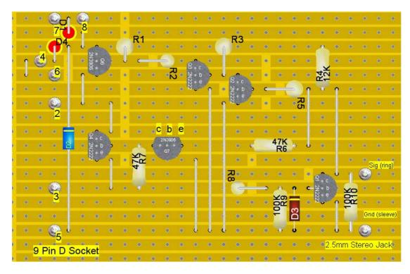
The layout was compressed to fit into an aluminium "u" box measuring 75x50x25mm.
